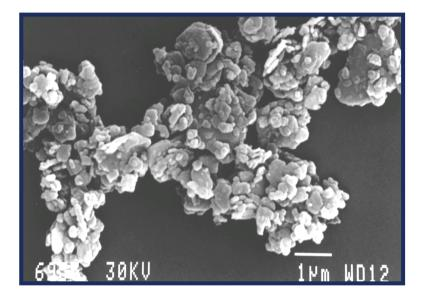
SEM and TEM Images showing the structure of Polarite (calcined kaolin).
