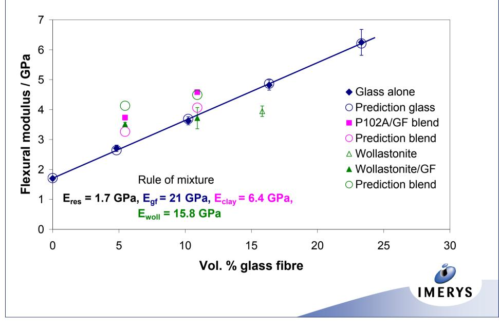
There is a linear variation in modulus with GF loading, in line with the predicted model.
