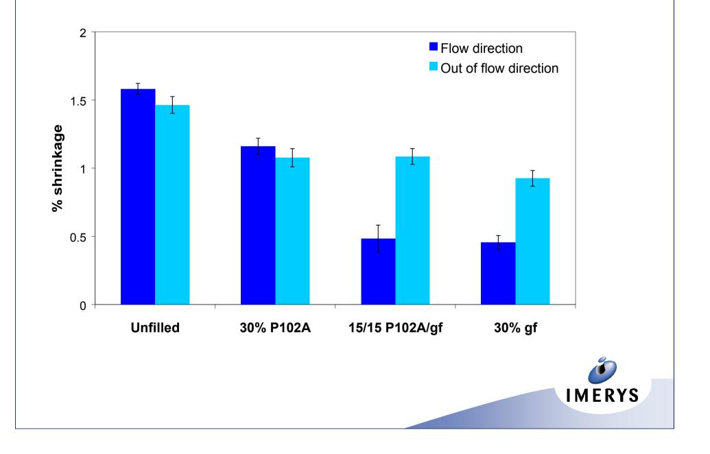
The addition of mineral and GF reduced the total shrinkage. The addition of 30 wt.% P102A gave similar shrinkage in both flow directions.
