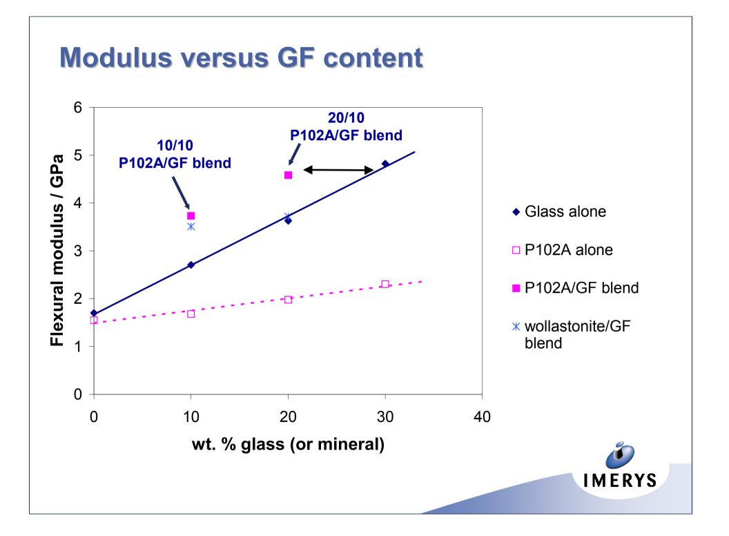
A 10/20 blend of P102A/GF gave the same modulus as a 20 wt.% GF.
