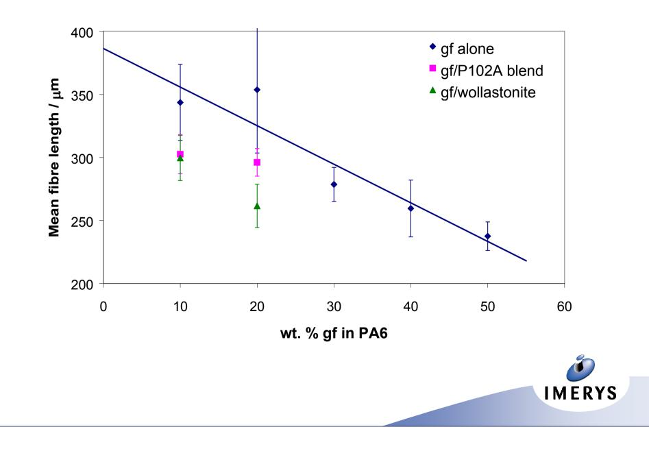
The average GF length decreases with increasing loading. At 10 wt.% mineral blends the fibre length is reduced by approximately 50  $\mu$ m. At 20 wt.% wollastonite it is reduced further by 50  $\mu$ m. The P102A GF length does not change. The deviation from the blend model for **wollastonite** can be explained in terms of attrition of the GFs, resulting in a lowering of the modulus.
